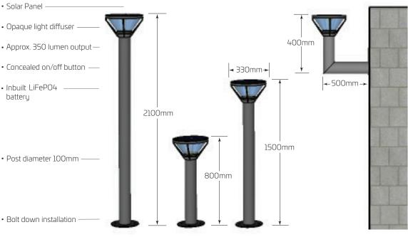
Suitable for inground, bolt-down or wall mount installation.
